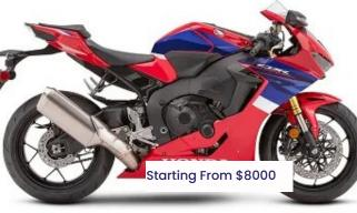
Engine: Standard Engine Type: Horizontal In-line Cylinders: 4 Engine Stroke: 4-Stroke Cooling: Liquid Valves:16 Valves per Cylinder: 4 Valve Configuration: DOHC Compression Ratio: 13:1 Starter: Electric Fuel Type: Gas Carburetion: Standard Fuel Injector: Yes Carburetor: No Carburetion Type: Fuel Injected Speed Governor: No Bore (mm/in): 76 / 2.99 Stroke (in/mm): 2.17 / 55 Displacement (cc/ci): 999.8 / 61 Fuel Injector Size (mm): 48
