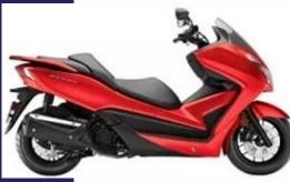
Engine Type: Single-Cylinder Cylinders: 1 Engine Stroke: 4-Stroke Cooling: Liquid Valves: 4 Valves Per Cylinder: 4 Valve Configuration: SOHC Bore (mm/in): 72 / 2.83 Stroke (mm/in): 68.5 / 2.7 Displacement (cc/ci): 279.2 / 17 Compression Ratio: 10.5:1 Starter: Electric Fuel Requirements: Regular Fuel Type: Gas Fuel Injector: Yes
