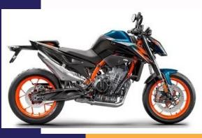
Engine: Standard Engine Brand Name: LC8C Engine Type: Parallel Twin Cylinders: 2 Engine Stroke: 4-Stroke Cooling: Liquid Valves: 8 Valves Per Cylinder: 4 Valve Configuration: DOHC Compression Ratio: 13.5:1 Starter Flectric Fuel Type: Gas Fuel Requirements: Premium Carburetion: Standard Carburetion Brand: Dell'Orto Fuel Injector: Yes Carburetor: No Carburetion Type: Fuel Injected Horsepower (bhp): 119.3 Bore (mm/in): 90.7 / 3.57 Stroke (in/mm): 2.71 / 68.8 Displacement (cc/ci): 889 / 54.2
