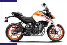
Engine: Standard Engine Brand Name: LC4c Engine Type: Single-Cylinder Cylinders: Engine Stroke: 4-Stroke Cooling: Liquid Valves: 4 Valves Per Cylinder: Valve Configuration: DOHC Starter: Electric Fuel Type: Gas Fuel Requirements: Premium Carburetion: Standard Carburetion Brand: Bosch Fuel Injector: Yes Carburetor: No Carburetion Type: Fuel Injected Horsepower (bhp): 30.8 Torque (Nm): 25 Bore (mm/in): 72 / 2.83 Stroke (in/mm): 2.41 / 61.2 Displacement (cc/ci): 249 / 15.2 FROM \$4500
