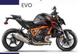
Engine: Standard Engine Brand Name: LC8 Engine Type: V Twin Cylinders: 2 Engine Stroke: 4-Stroke Torque RPM: 7000 Cooling: Liquid Valves: 8 Valves Per Cylinder: 4 Valve Configuration: DOHC Starter: Electric Fuel Type: Gas Fuel Requirements: Premium Carburetion: Standard Carburetion Brand: Keihin Fuel Injector: Yes Carburetor: No Carburetion Type: Fuel Injected Horsepower (bhp): 188 Torque (Nm): 145 Bore (mm/in): 110 / 4.33 Stroke (in/mm): 2.8 / 71 Displacement (cc/ci): 1350 / 82.4
