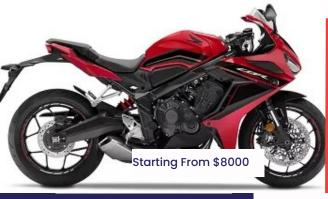
Engine Type: In-line Cylinders: 4 Engine Stroke: 4-Stroke Cooling: Liquid Valves:16 Valves per Cylinder: 4 Valve Configuration: DOH Compression Ratio: 11.6:1 Starter: Electric Fuel Type: Gas Carburetion: Standard Fuel Injector: Yes Carburetor: No Carburetion Type: Fuel Injected Speed Governor: No Bore (mm/in): 67 / 2.64 Stroke (in/mm): 1.81 / 46
