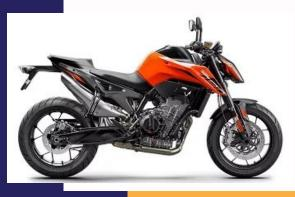
Engine: Standard Engine Brand Name: LC8C Engine Type: Parallel Twin Cylinders: 2 Engine Stroke: 4-Stroke Torque RPM: 8000 Cooling: Liquid Valves: 8 Valves Per Cylinder: 4 Valve Configuration: DOHC Starter Flectric Fuel Type: Gas Fuel Requirements: Premium Carburetion: Standard Carburgtion Brand: Bosch Fuel Injector: Yes Carburetor: No Carburetion Type: Fuel Injected Horsepower (bhp): 105 Torque (Nm): 87 Bore (mm/in): 88 / 3.46 Stroke (in/mm): 2.59 / 65.7 Displacement (cc/ci): 799 / 48.7
