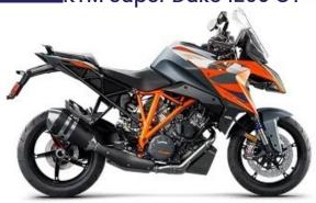
Engine Type: V Twin Cylinders: 2 Engine Stroke: 4-Stroke Cooling: Liquid Valves: 8 Valves Per Cylinder: 4 Valve Configuration: DOHC Compression Ratio: 13.2:1 Starter: Electric Fuel Type: Gas Fuel Requirements: Premium Carburetion: Standard Carburetion Brand: Keihin Fuel Injector: Yes Carburetor: No Carburetion Type: Fuel Injected Horsepower (bhp): 175 Torque (Nm): 141 Bore (mm/in): 108 / 4.25 Stroke (in/mm): 2.8 / 71 Displacement (cc/ci): 1301 / 79.4 Fuel Injector Size (mm): 56
