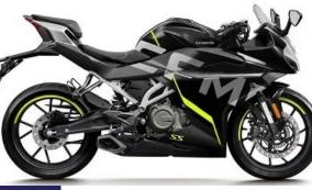
Engine: Standard Engine Type: Single-Cylinder Cylinders: 1 Engine Stroke: 4-Stroke Horsepower RPM: 8750 Torque RPM: 7250 Cooling: Liquid Valves: 4 Valves Per Cylinder: 4 Valve Configuration: DOHC Starter: Electric Fuel Type: Gas Fuel Requirements: Regular Carburetion: Standard Carburetion Brand: Bosch Fuel Injector: Yes Carburetor: No Carburetion Type: Fuel Injected Horsepower (bhp): 29 Torque (Nm): 25.4 Bore (mm/in): 78/3 Stroke (in/mm): 2.4 / 61.2 Displacement (cc/ci)|: 292/17.8
