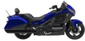
Engine: Standard Engine Type: Horizontally Opposed Cylinders: 6 Engine Stroke: 4-Stroke Cooling: Liquid Torque RPM: 6250 Valves:12 Valves per Cylinder: 2 Valve Configuration: SOHC Compression Ratio: 9.8:1 Starter: Electric Fuel Type: Gas Carburetion: Standard Fuel Injector: Yes Carburetor: No Carburetion Type: Fuel Injected Bore (mm/in): 72/ 2.92 Stroke (in/mm): 2.8 / 71 Displacement (cc/ci): 1832 / 111.8 US Miles Per Gallon (Combined): 34 Kilomenter (Combined): 6.9 Fuel Injector Size (mm): 40
