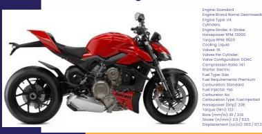
Engine: Standard Engine Brand Name: Desmosedici Stradale Engine Type: V4 Cylinders: Engine Stroke: 4-Stroke Horsepower RPM: 13000 Torque RPM: 9500 Cooling: Liquid Valves: 16 Valves Per Cylinder: Valve Configuration: DOHC Compression Ratio: 14:1 Starter: Electric Fuel Type: Gas Fuel Requirements: Premium Carburetion: Standard Fuel Injector: Yes Carburetor: No Carburetion Type: Fuel Injected Horsepower (bhp): 208
