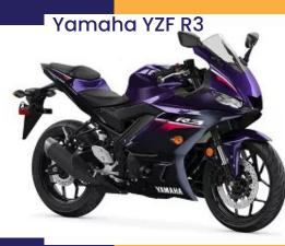
**Engine: Standard** Engine Type: Parallel Twin Cylinders: 2 Engine Stroke: 4-Stroke Cooling: Liquid Valves:8 Valves per Cylinder: 4 Valve Configuration: DOHC Compression Ratio: 11.2:1 Starter: Electric Fuel Type: Gas Fuel requirements: Regular Carburetion: Standard Fuel Injector: Yes Carburetor: No Carburetion Type: Fuel Injected Bore (mm/in): 68 / 2.68 Stroke (in/mm): 1.74 / 44.1 Displacement (cc/ci): 321 / 19.6
