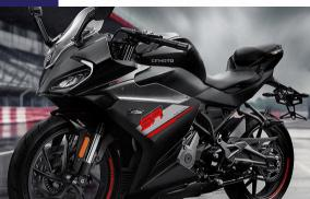
Engine Type: Single-cylinder, liquid-cooled, DOHC Displacement: 249 cc Bore x Stroke: 72 x 61.2 mm Maximum Power: 20.5 kW / 9750 rpm Maximum Torque: 22 Nm / 7250 rpm
